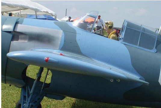
There's no washout and no incidence in Dave Deschenes' Wildcat—typical of constant-chord dive bombers.
