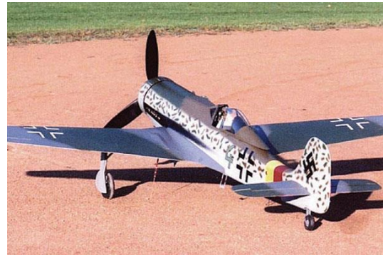
The glider-like wing of the author's 114-inch span Focke-Wulf Ta 152H requires washout for stability. The aircraft would be uncontrollable without it.
