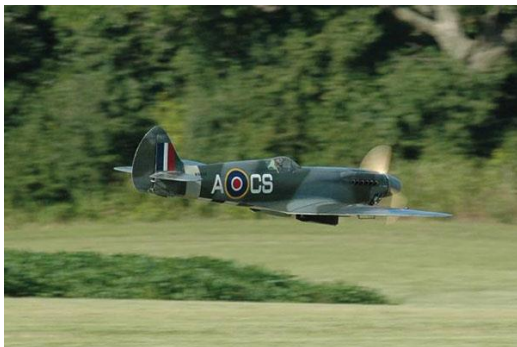
Despite its thin, pointed wingtips, Dave Szabo's Spitfire has excellent handling in part because of 2.5° of washout—roughly the same as the full-scale Spitfire. A low pass before a chandelle is shown here.
