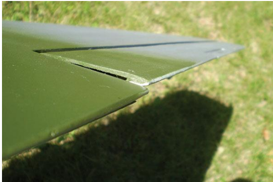
Washout can be added after construction by slightly raising both ailerons. This is recommended for the maiden flights of a new model.
