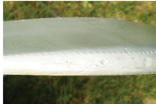
Washout in the Howard Pete's wingtip is formed by shaping the LE in the outer rib bay.
