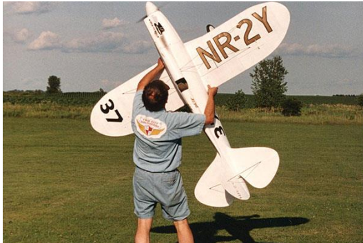
The author's Howard Pete has washout in only the last rib bay—enough for a nearly constant chord wing
