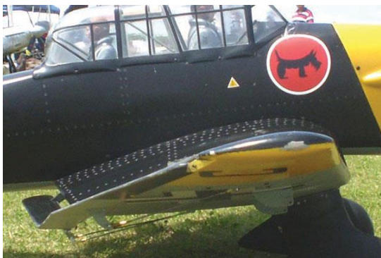
Leo Spychalla's Zirol Stuka has a gentle stall despite its pointed wings. The wings have 4° of washout, starting outboard of the landing gear.
