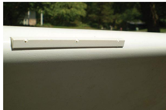
A 90° sharp-edge stall strip is added to the LE of the Grumman Lynx to lower the stall angle in the root area of the wing. This alternative to washout also works when inverted.
