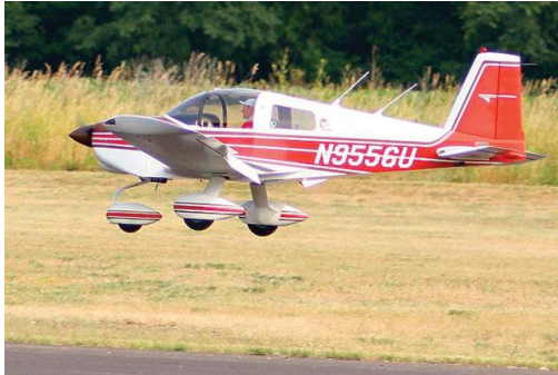
The author's 1/3-scale Grumman Lynx has a constant chord wing with no washout. It instead uses Hoerner wingtips and stall strips, which are effective.
