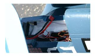
All of the power system components should be inspected. The battery should be fully charged and in good shape. The transmitter and receiver batteries need to be fully charged and need to hold that charge. The ESCs and BEC must operate within their stated limits.
