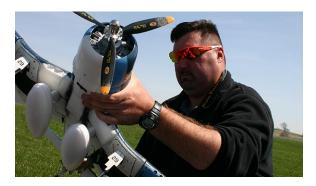
Inspecting the propellers/blades is essential. Cracks or chips could lead to disaster. Replace any that show signs of wear, and make sure you have extras available.
