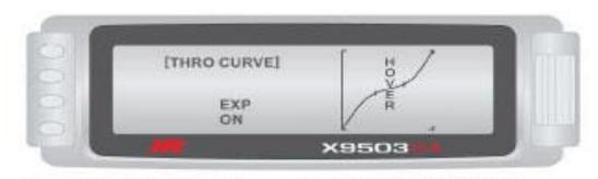
If over-controlling the throttle is a problem, some pilots find it helpful to flatten the throttle curve around the hover throttle setting to dampen the throttle response.
