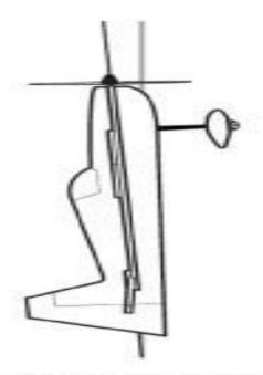
Most models lock into a more stable hover when the fuselage is held a couple degrees past vertical (tilted slightly toward the canopy) to compensate for the propwash striking the underside of the stab.
