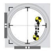
To avoid aggravating the pendulum effect, larger corrections will require returning the control stick past neutral into a brief opposite input to halt the response.
