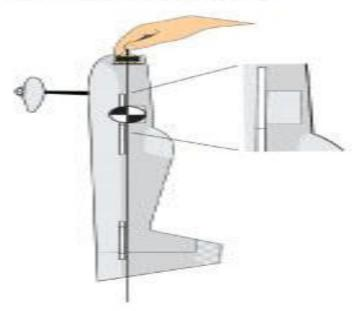
Check the vertical balance of your smaller 3D models by supporting them from the propeller shaft. When possible, move things toward the top of the fuselage to achieve a better vertical balance and a more stable, less-demanding hover.
