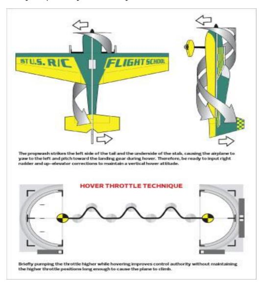
Enter a hover by reducing power and airspeed, then quickly pull to vertical while simultaneously adding power, right rudder, and alleron to counter proposash and torque.
