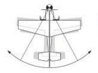
To avoid over-controlling, try to limit your rudder and elevator corrections to small brief humps or jabs when working to keep the fuselage vertical during hover.
