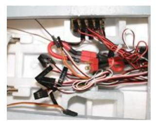
Eleven servos and an onboard LED lighting system overtax the speed control's BEC.
