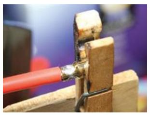
A good soldered joint between the wire and 6mm bullet will handle a lot of current. Note that there is no excess solder running all over the outside of the bullet and the joint is shiny clean.
