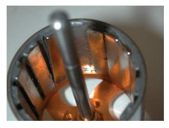
Poorly constructed motors can throw magnets and cause extreme current spikes that will destroy a speed control. Quality Matters
