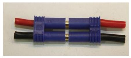
An improper extension made by jamming a bullet into the EC5 connectors. Great connectors ruined by a bad idea.
