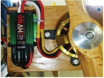
Note the securely attached speed control for this big power system and how the connections are well insulated and secured. Short wire runs and a protective grommet in the firewall, where the wires pass through, ensures no shorts over time.
