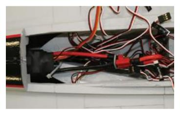
The speed control in this foam jet is jammed into the nose, so it's fully insulated and gets no cooling air. With the heavy load from the motor and too many servos, this will overheat and die quickly.
