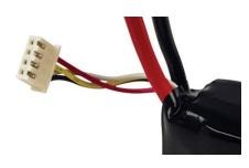
The XH balance connector has become the most common connector found on batteries in the US. E-flite and ElectriFly are examples of brands that use this plug.
